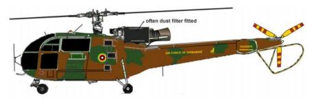
the tail end plates and the tail boom has the yellow AIR FORCE titles with bird. The tail rotor colours are standard yellow with red stripes and a yellow-black striped tail bar. On the nose, a pair of wire antennas is common.
