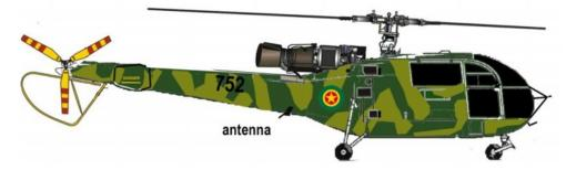
It has the basic Alouette configuration. The tail rotor colours are standard yellow with red stripes and a yellow tail bar. The main rotor tips are bright red. Add a small blade antenna on the starboard side at the tail boom and a pair of wire antennas on the nose. The danger marking in yellow is on each tail fin plate. (It is unknown if a roundel was set aft of the nose gear on the belly).
