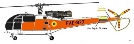
white with bright orange trim (approx. FS12510). The horizontal tail stabilizer and the tail fin plates are also orange. The tail rotor colours are standard yellow with red stripes and a yellow tail bar. The main rotor tips are bright red. The two tail fin plates have the national flag, trim the provided stripe decal.
