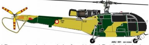
around camouflage of olive drab and sand. The rear engine exhaust cover is also often painted sand. The tail rotor bar is yellow and the tail rotor yellow with red stripes. The red danger marking is at the end of the tail boom. There are a few blade antennas situated at the nose and a pair of wire antennas running from the tail bar to the main gear legs.
