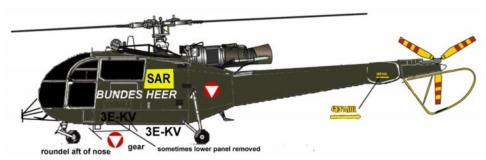
cabin panel has been removed (so a gap is there). The tail rotor colours are standard yellow with red stripes and a yellow tail bar with black stripe. The main rotor tips are bright red. On the nose rods with antennas/ mirrors are fitted.
