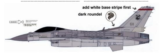
[A] F-16C Block 52 of the Singapore Air Force coded 611 of no.140 squadron "Osprey". It has the Pratt and Whitney F100 engine with standard intake.
