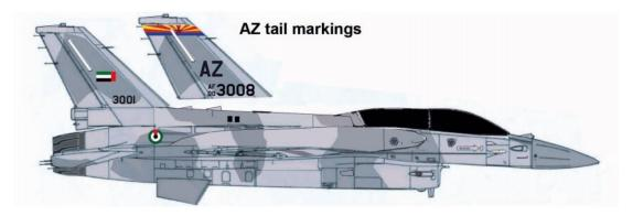
[B] F-16**F** Block 60 of the United Arab Emirates Air Force coded 3001. It has the GE F110 engine with bigger MCID intake. IFF antennas fitted on nose. The long fuselage spine fairing contains various systems and includes the thicker tail base fairing.
