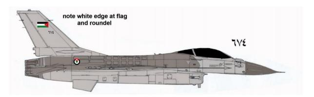
[A] F-16 ADF of the Jordanian air force coded 674, set in arab numbers. (ex-US ANG). (other codes also provided). It has the Pratt and Whitney F100 engine with standard intake. IFF antennas fitted on nose. Note ADF fairing at tail base (both sides) and short tail base without parachute housing.
