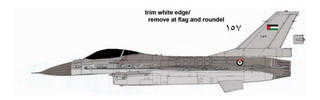
[B] F-16AM (MLU) of the Jordanian air force coded 157 (c/n 6H-120/M13-454 was the ex-Belgian F-16AM FA120). It has the Pratt and Whitney F100 engine with standard intake. IFF antennas on nose.
