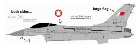
[A] F-16C Block 40 of the Royal Bahraini Air Force coded 109 serial 90-0032 was delivered from 1990. It has the Pratt and Whitney F100 engine with standard intake. IFF antennas on nose and capable to fire AMRAAM missiles. It is probable that structural stiffeners were mounted on the upper mid fuselage.
