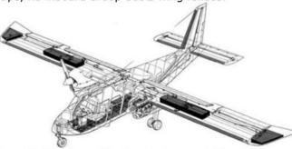
Length 10,86 m with standard nose. Later versions length of 12,20 m with extended radar nose.
