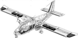
Length 10,86 m with standard nose. Later versions length of 12,20 m with extended radar nose.
