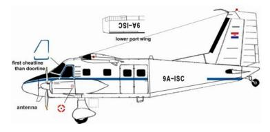
The leading edges of wing (full span), horizontal stabilizers and tail are black. The cheatline decals need to be trimmed to correct lengths. The registration is below the port wing, unclear if also on top of the wing. Spinners are white, propeller blades light gull grey with yellow tips. A wire antenna runs from tail to forward fuselage.
